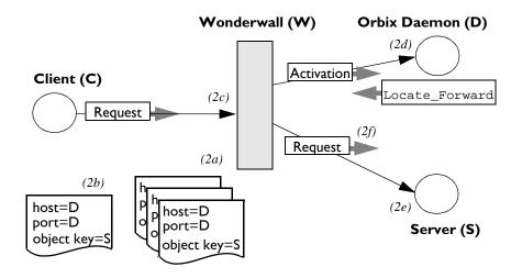
Figure 4.4: Establishing a Connection Through Wonderwall
