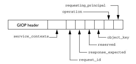
Figure 3.3: The Format of a Request Message Header
