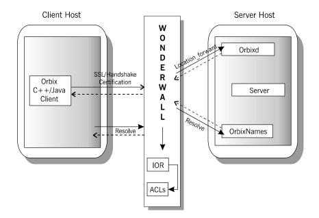
Figure 6.5: A Partially Secure Configuration
