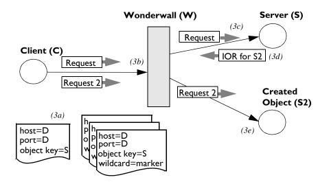
Figure 4.5: Establishing a Connection to a New Object Through Wonderwall
