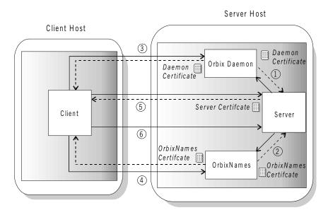
Figure 6.3: Running the Banking Application with SSL Security
