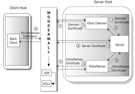
Figure 6.4: A Fully Secure Banking Application
