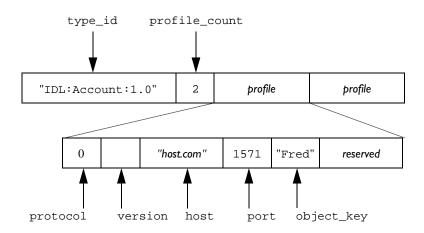
Figure 3.1: The Format of an Interoperable Object Reference and Profile
