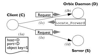
Figure 4.3: Establishing a Normal Connection
