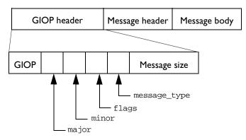
Figure 3.2: The Format of a GIOP Message and Message Header
