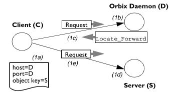
Figure 6.3: Establishing a Normal Connection
