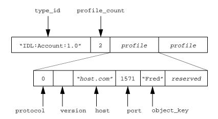
Figure 5.1: The Format of an Interoperable Object Reference and Profile
