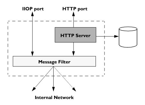
Figure 2.2: Internal Architecture of the Wonderwall Proxy Server
