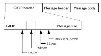
Figure 5.2: The Format of a GIOP Message and Message Header
