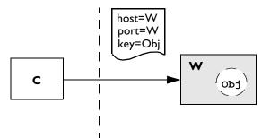
Figure 6.1: Apparent Location of Object, in Wonderwall Proxy Server
