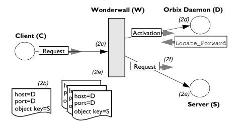
Figure 6.4: Establishing a Connection Through Wonderwall
