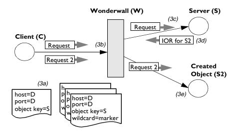
Figure 6.5: Establishing a Connection to a New Object Through Wonderwall
