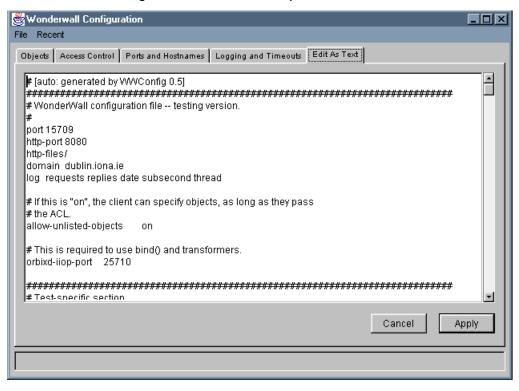
Figure 3.8: Wonderwall GUI Configuration Tool Edit As Text Window
