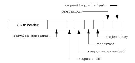
Figure 5.3: The Format of a Request Message Header
