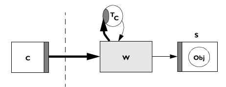
Figure 7.2: Encrypted Link Using Wonderwall
