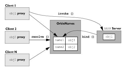
Figure 3.1: Example of Typical OrbixNames Usage
