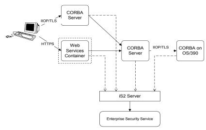
Figure 1 Orbix Security Framework Architecture
