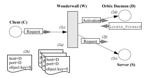
Figure 4.4: Establishing a Connection Through Wonderwall
