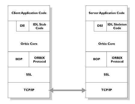
Figure 6.1: The Role of SSL in Orbix Client/Server Communications
