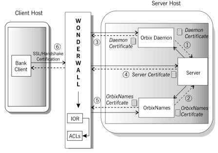
Figure 6.4: A Fully Secure Banking Application
