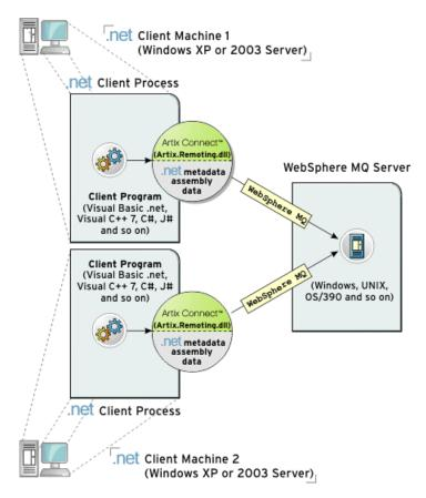
Figure 25: Typical Deployment Scenario
