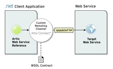
Figure 2: .NET client invoking on SOAP over HTTP Web Service
